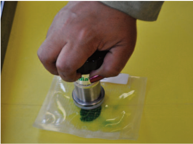
Step 3. Rub the bag with a handheld homogenizer or blunt instrument (pencil, scissors handle, etc.) to crush the tissue and produce an extract.
