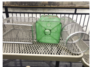
Figure 17. Three different types of crayfish traps. The middle one is collapsible and easy to pack into a distant stream or pond.
